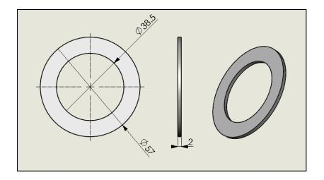
61056 Camshaft Grease Seal
