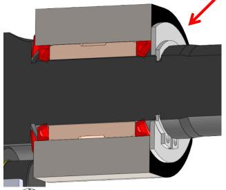
The direction of the grease seals in the anchor bracket is important as well as the position of the beveled washer between the anchor bracket and camshaft head.
