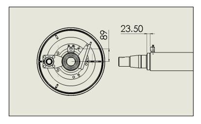
Pole wheel at 178mm PCD Face of sensor block 23.5mm from large bearing shoulder Bolt on ABS block (as shown above) is positioned 90 degrees to camshaft. Weld on style is 180 degrees to camshaft and is in line with hole in anchor bracket.
