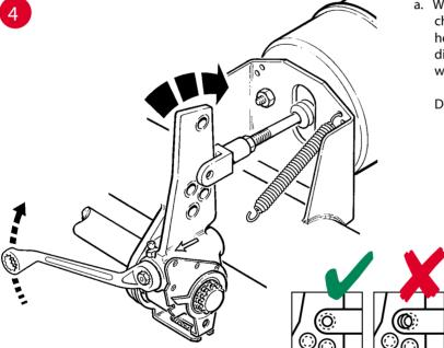
a. Wind the ASA into the clevis on the brake chamber piston rod by rotating the hexagon nut on the ASA in a clockwise direction until the hole in the ASA coincides with the holes in the clevis.
