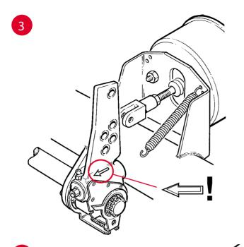
a. Fit the ASA onto the camshaft, so that the arrow on the housing points in the direction of the application of the ASA, and the control arm end mates with the anchor bracket.
