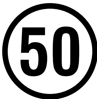
Figure 21: Model speed disc for an agricultural tractor, self-propelled agricultural machine, agricultural trailer or piece of interchangeable towed equipment showing a maximum design speed of 50 km/h.
