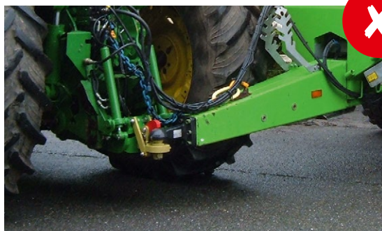
Figure 18: Incorrectly fitted safety chain. (Image courtesy of Dromone Engineering)
