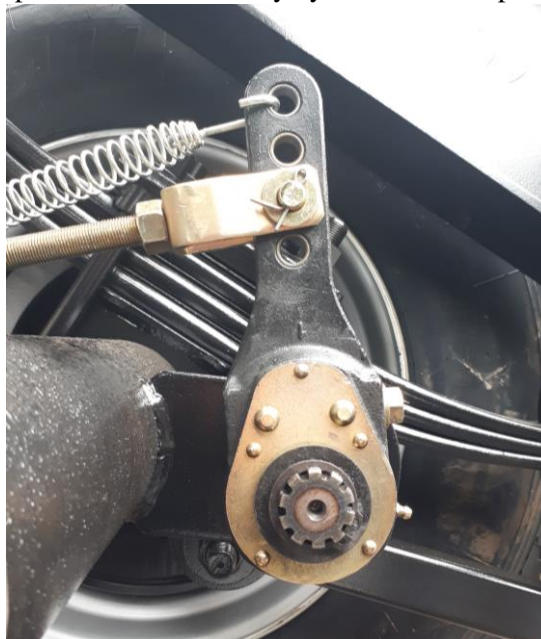
Figure 14. Clevis head pin and split washer fitted.
