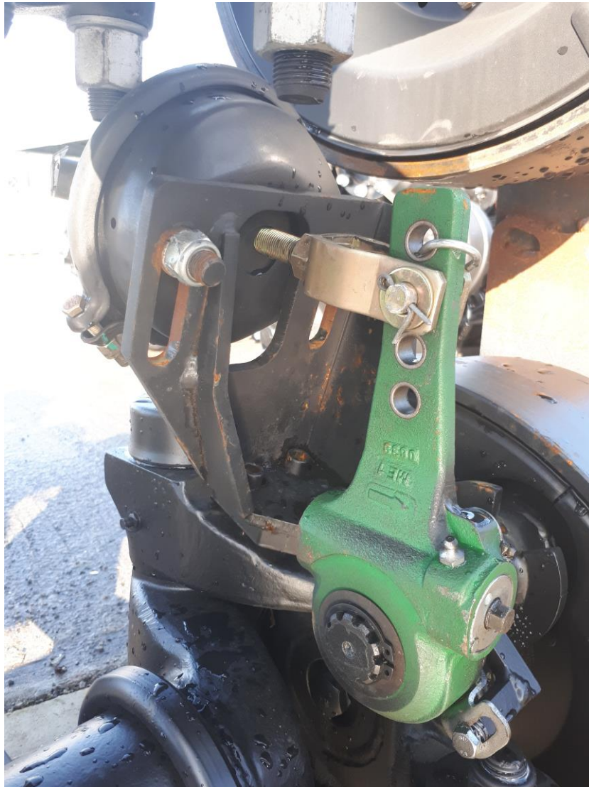
Figure 26: Service brake chamber mounted with a straight autoslack at 178mm lever length.
