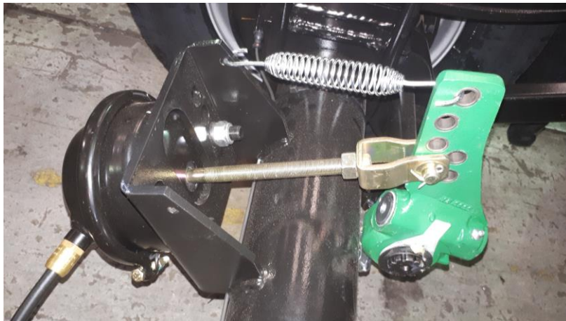
Figure 21: Brake chamber, automatic slack adjuster, wear indicator, and return spring fitted to axle.
