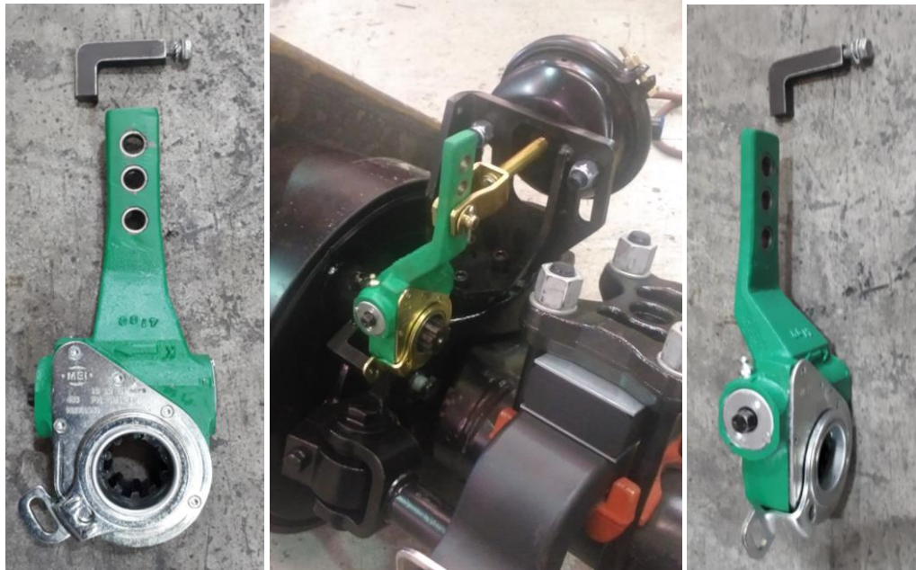
Figure 6. Offset automatic slack adjuster shown fitted to axle with “L” control arm.
