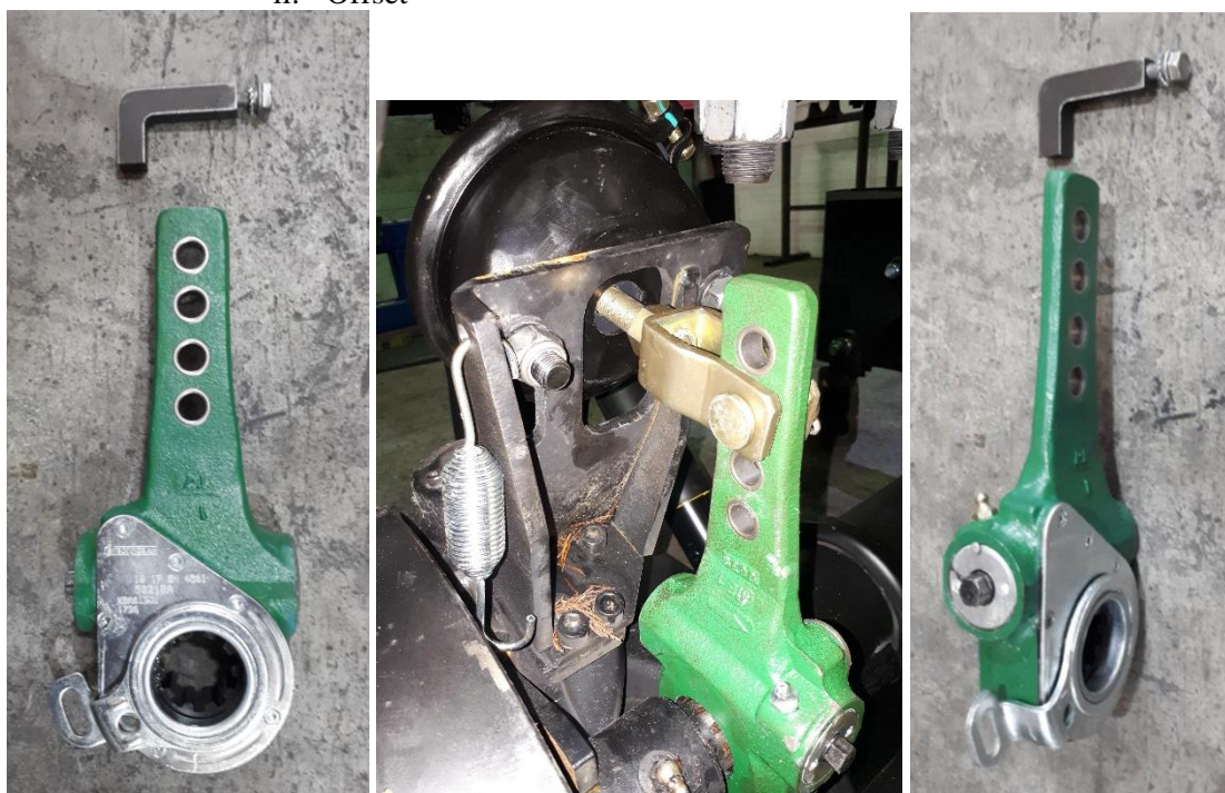
Figure 5. Straight automatic slack adjuster shown fitted to axle with “L” control arm.
