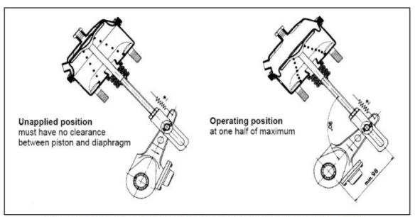
Slack adjuster and push rod at 90° when brake chamber at half stroke.
