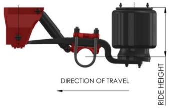
On an air suspension Ride Height is the distance from the centre of the axle to the underside of chassis. With Air Suspension this height is the same whether laden or unladen.
