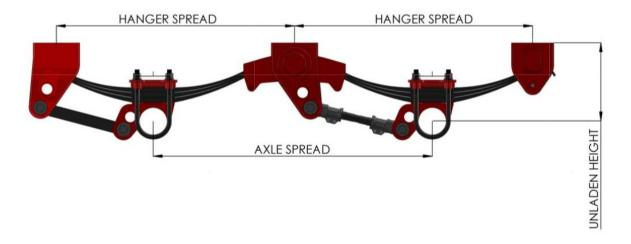
On a mechanical suspension the ride height is the distance from the centre of the axle to the underside of the chassis but the height is different if the suspension is laden or unladen as the mechanical spring deflects with weight.
