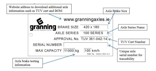
Go to the 'Search' bar on the main Granning website. Put in the axle serial number and the information on that axle will appear. For example type in axle serial number E16F07067
