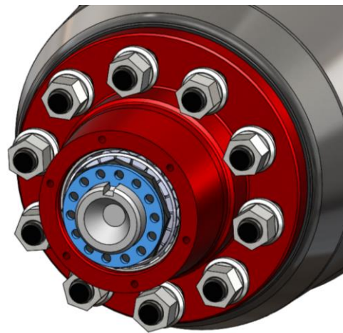
Then remove the tab washer and the lock washer.
