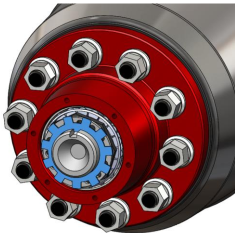
Then remove the tab washer and the lock washer.
