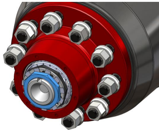
Straighten locking tab, then undo and remove locknut.
