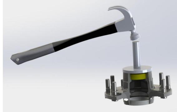
Outer bearing cone being fitted
