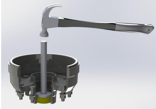
Outer bearing cone being removed.
