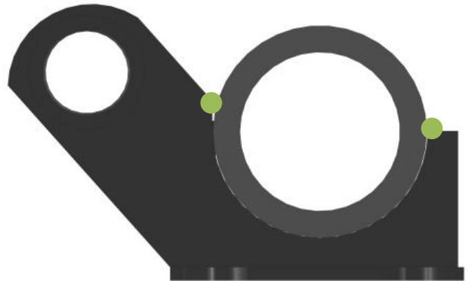
36146 Axle seat – Weld details
