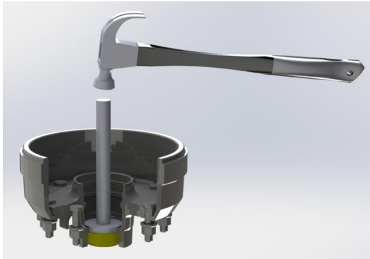
Outer bearing cone being removed.
