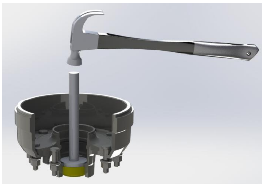
Outer bearing cone being removed.
