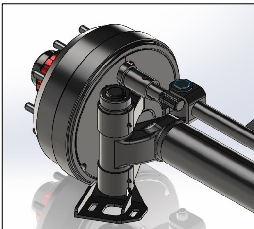
860 "A" Series – No grease nipple in the track rod bolt and steer angle limiting bolt threaded into the beam knuckle.
