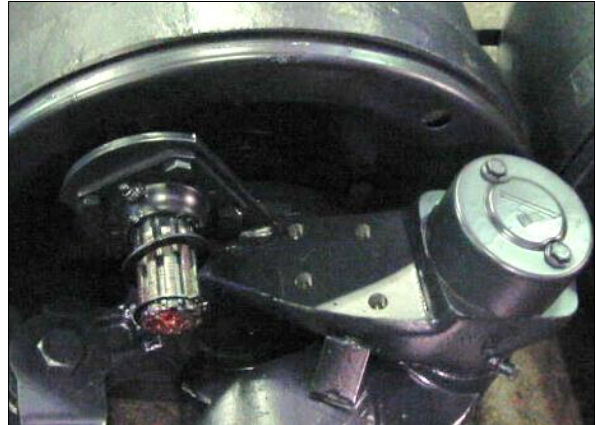
100 & 300 "F" Series – ACB holes tapped directly into steer axle knuckle.
