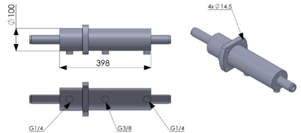
37293- Self steer hydraulic ram. Hydraulic ram integrated with track rod. Used to lock and unlock steer axle.
