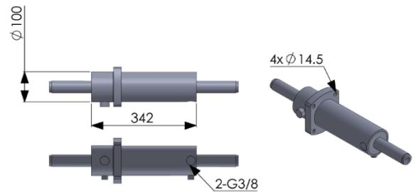
37253- Forced steer hydraulic ram. Hydraulic ram integrated with track rod.
