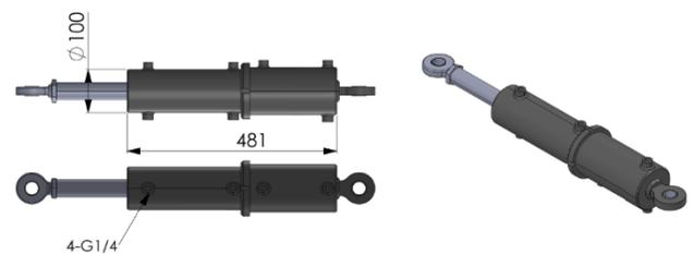
37178- Self steer hydraulic ram that can be piped for forced steer. Separate from track rod. 16T steer.
