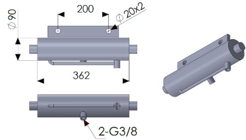
37179- Self steer hydraulic ram. Separate from track rod. Used to lock and unlock steer axle.
