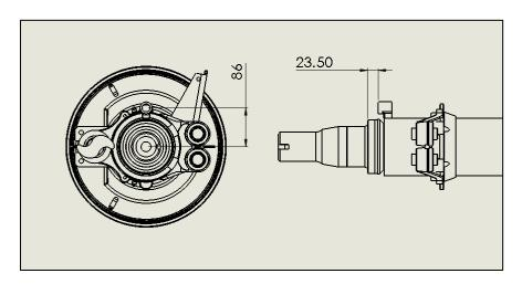
Centre of the ABS sensor is 86mm from centre of the axle Face of sensor block 23.5mm from large bearing shoulder Weld on ABS block (as shown above) is positioned 90 degrees to camshaft.
