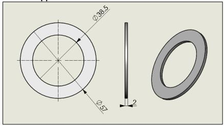
61056 - Camshaft Grease Seal
