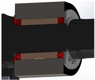
The direction of the grease seals in the anchor bracket is important as well as the position of the beveled washer between the anchor bracket and camshaft head.
