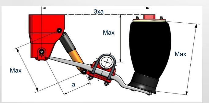
It is important is to understand that the hanger bracket height is related to air spring pedestal. You cannot change one without the other.
