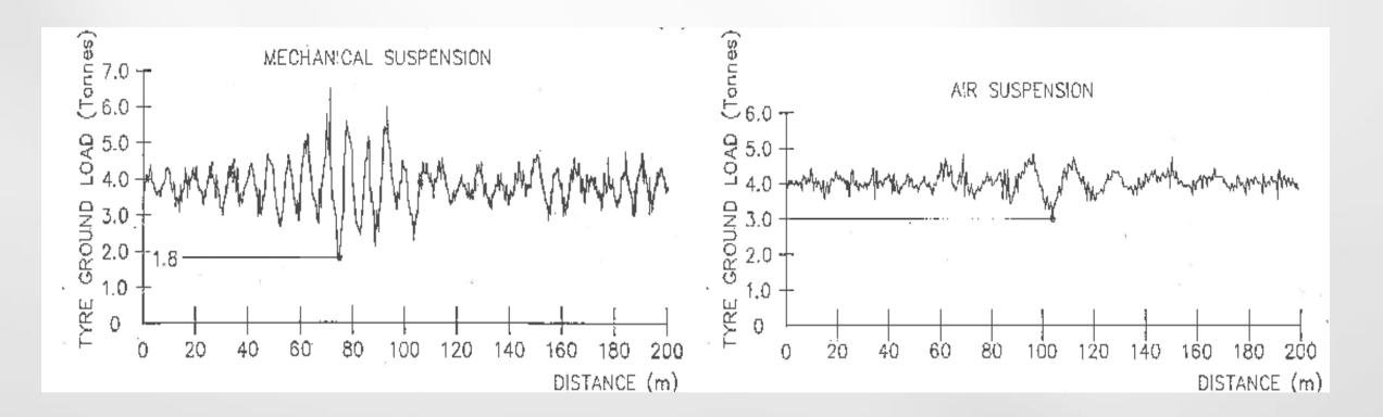
The two graphs are actual tire ground contact load traces measured on Air and Mechanical Suspensions.
