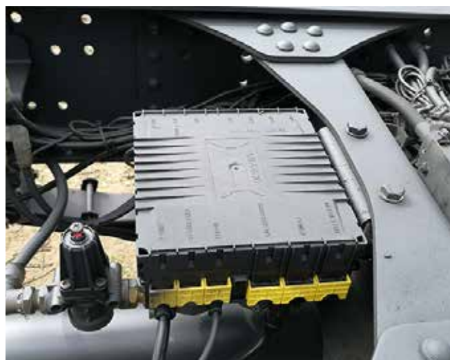
Independent EBS system fitted to truck additional axle
