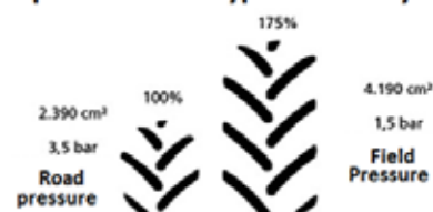
Tyre footprints and ground pressure with typical radial tyre
