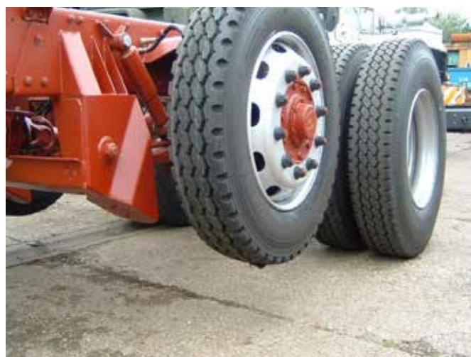
Mid axle installation, axle lifted.
