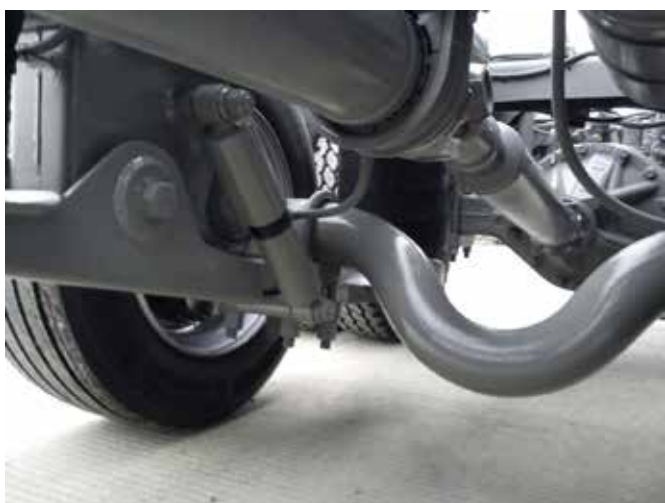
Mid axle showing Drop Centre Tube to avoid prop shaft
