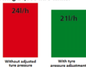
Fuel consumption of 260 hp tractor towing 24,000 litre tanker
